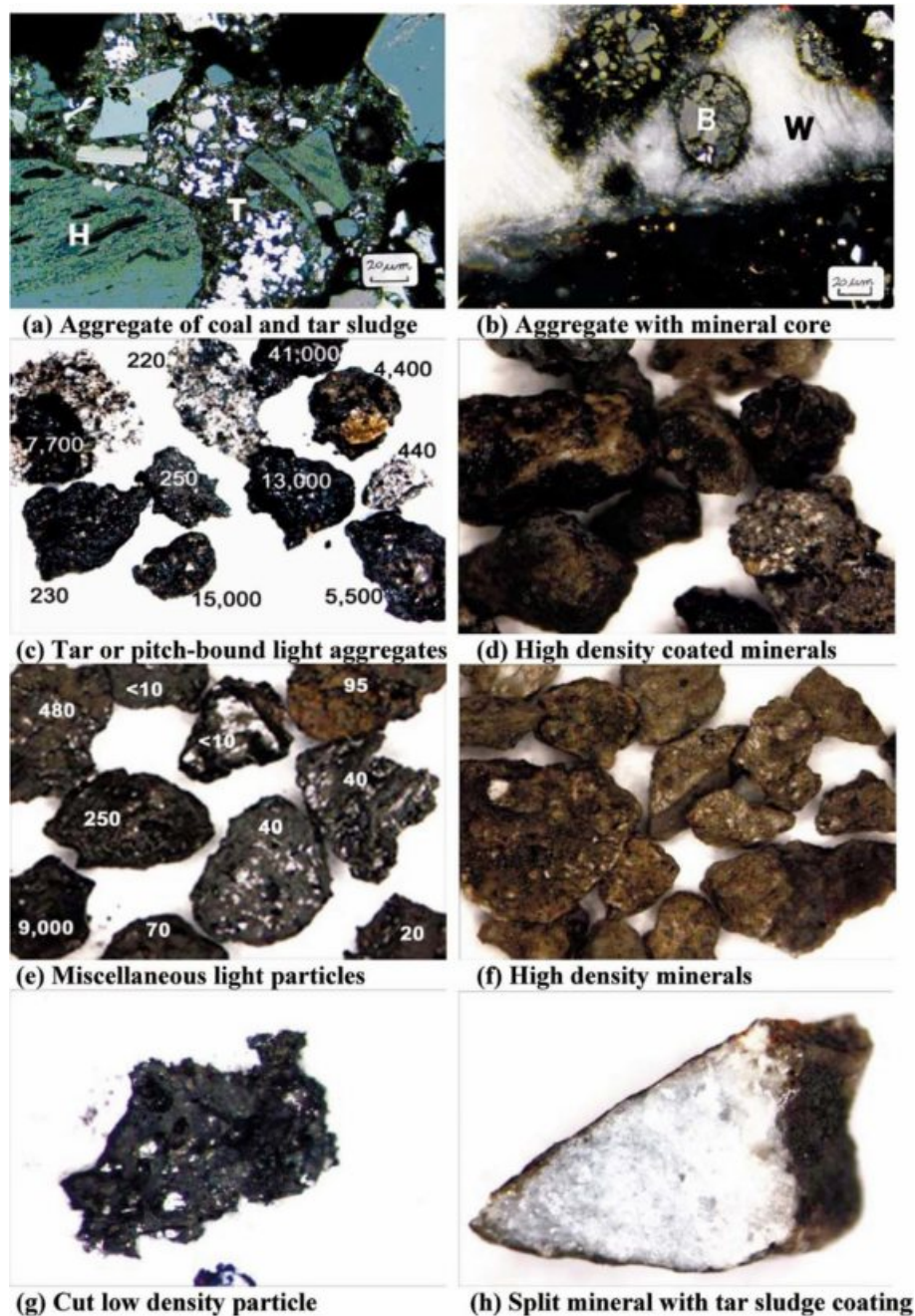
Fig. 1. Microscopic images of black carbonaceous aggregates or mineral matter coated with black carbonaceous matter collected from native soil near a coke plant. Reprinted with permission from Ahn et al. (2005). Copyright (2009) John Wiley and Sons.
