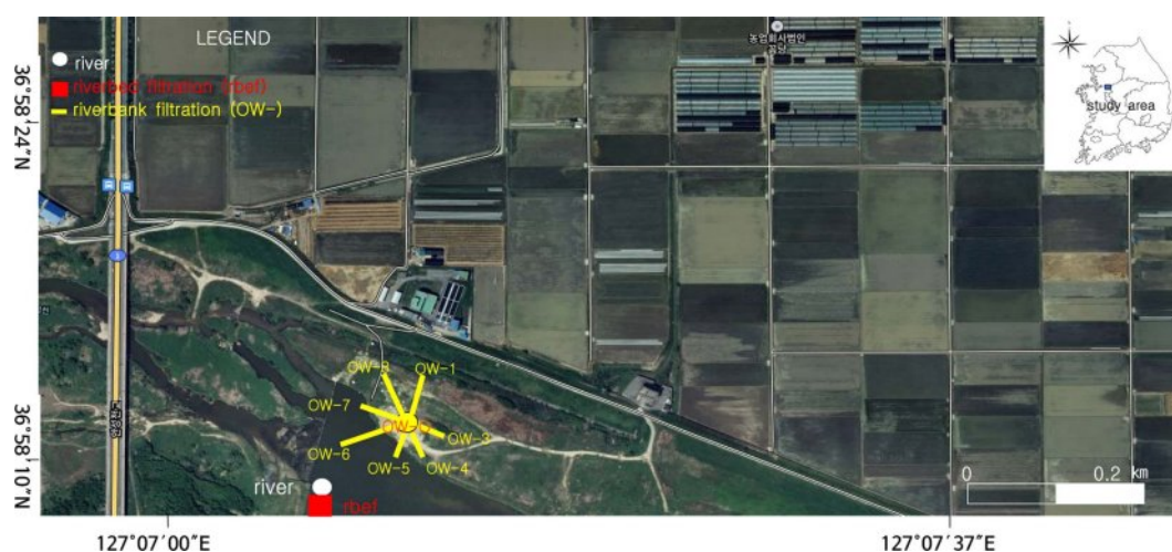
Fig. 3. Location map of the study area (Anseong): riverbed filtration (rbef) and riverbank filtration horizontal wells (OW-#).
