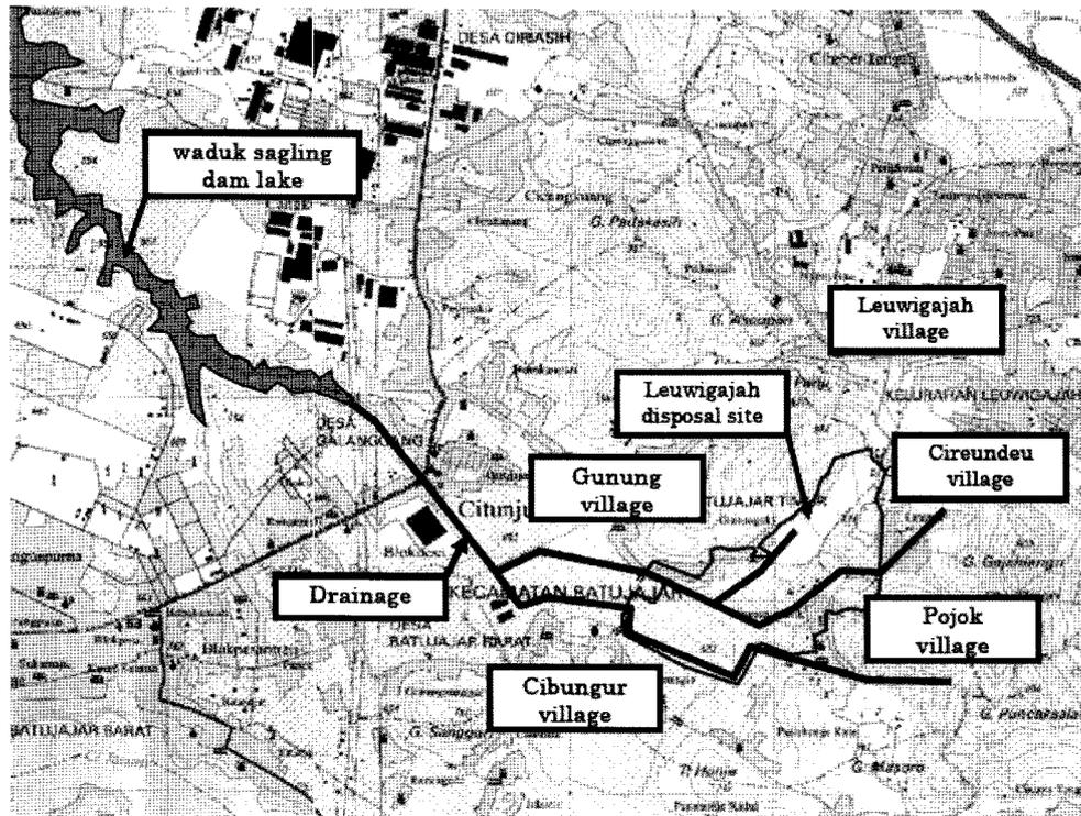
Fig. 11. Hydrological distribution around Leuwigajah landfill (Source: Yachiyo Engineering, 2009).
