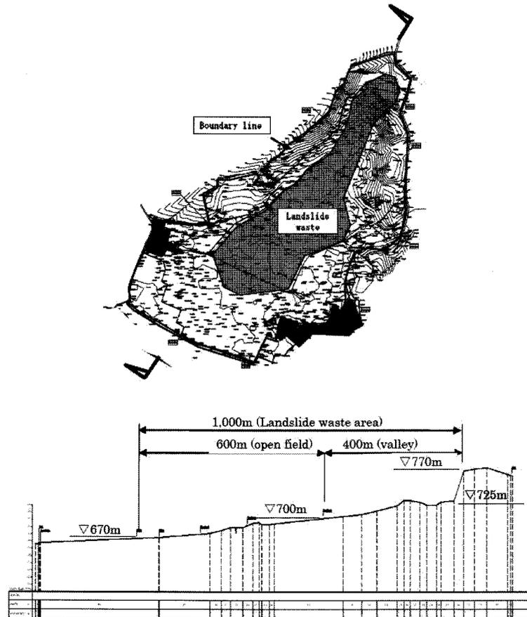
Fig. 10. Topographic condition of Leuwigajah landfill (Source: Yachiyo Engineering, 2009).
