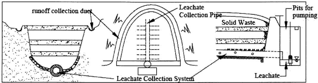
Fig. 12. Semi-aerobic landfill system.
