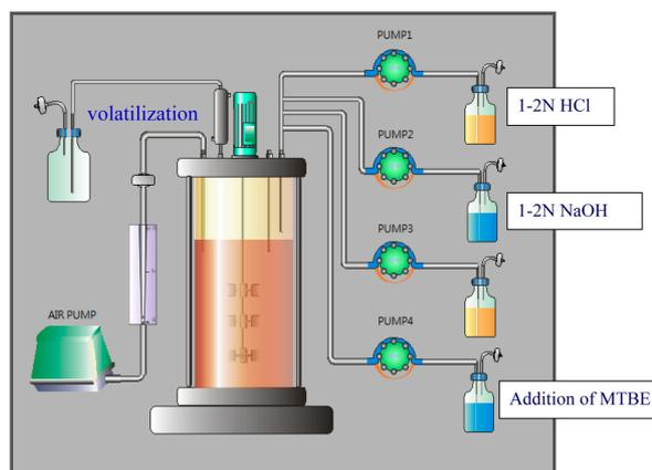
**Fig. 2.** The configuration of the bioreactor.
