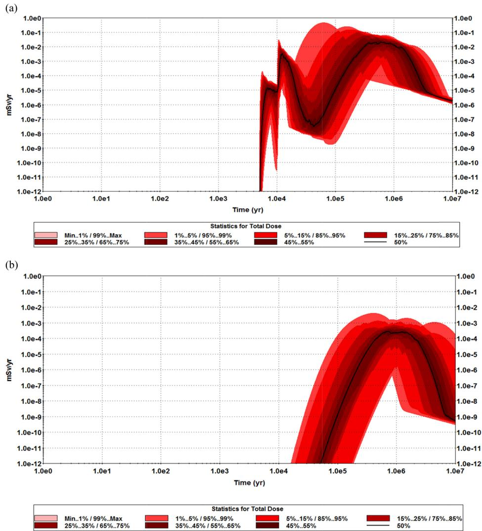
Fig. 8. Result from the probabilistic safety assessment for the well scenario, (a) rock cavern disposal facility and (b) near surface disposal facility.
