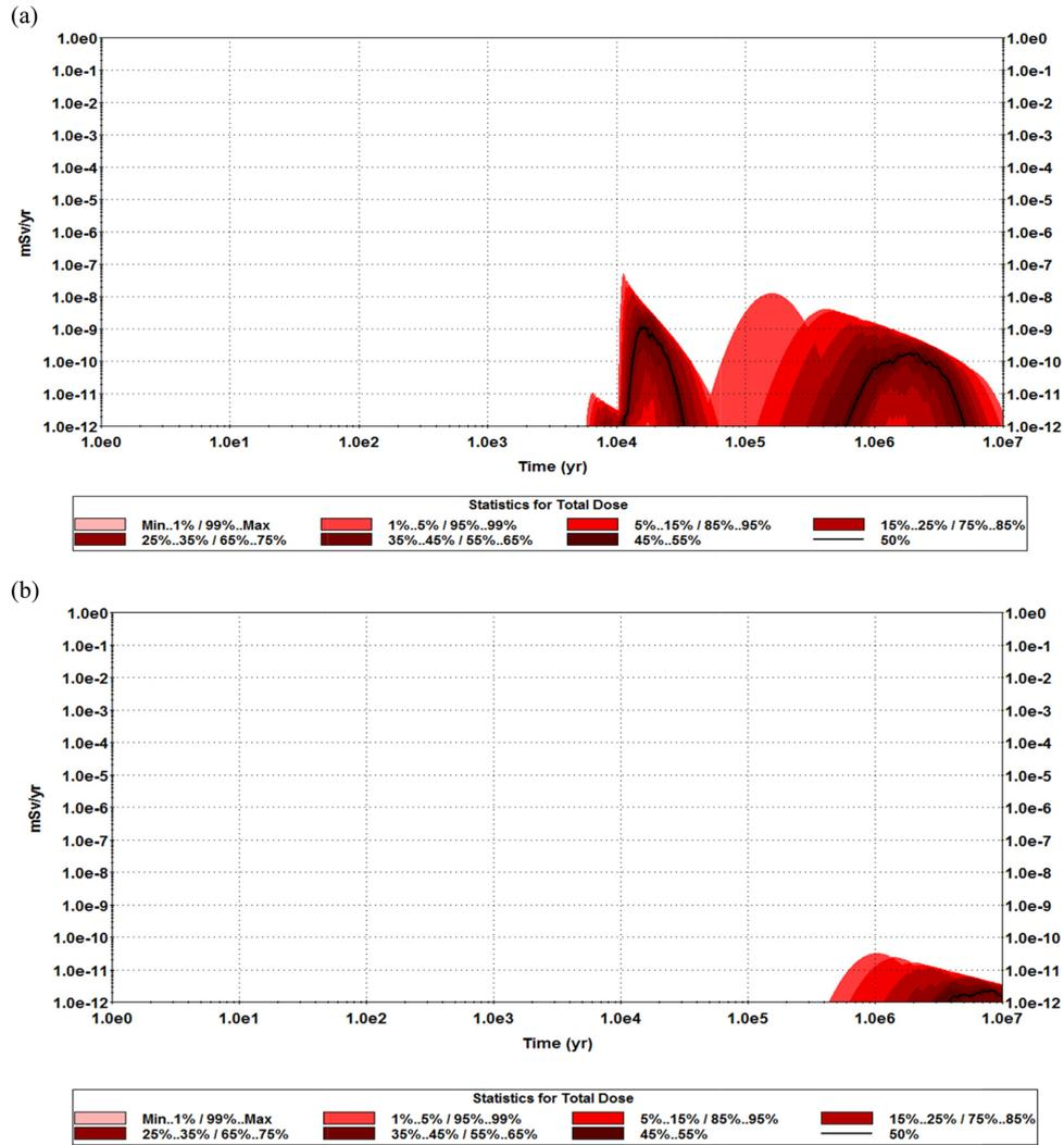
Fig. 6. Results from the probabilistic safety assessment for the normal scenario, (a) rock cavern disposal facility and (b) near surface disposal facility.
